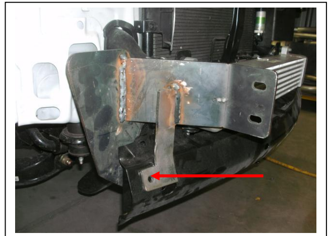
Figure 2: Drill top of bumper support to 10mm.
