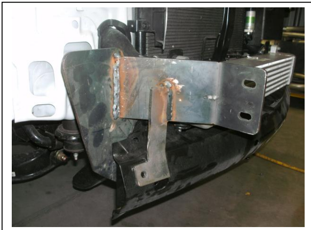
Figure 1: Mount between chassis and bumper support.
